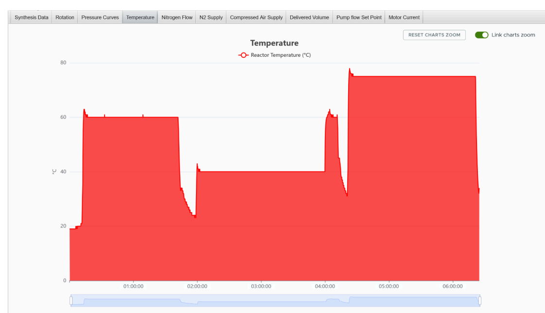
Figure 3. Temperature curve of the one-pot synthesis of Rufinamide
